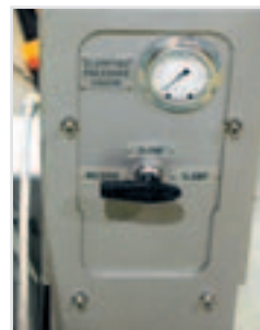
Screen-clamping system, with single-point, pneumatic control, speeds screen-changing operations
