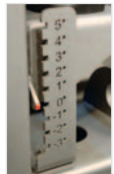
Bed-angle indicator aids accurate adjustment of basket angle
