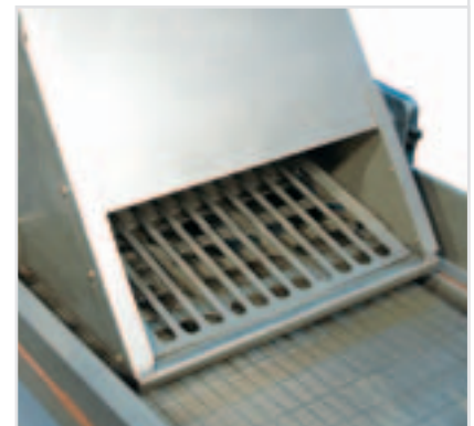
Gumbo slide design minimizes gumbo buildup.
