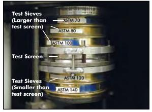
ASTM sieves mounted on Rotap with the test screen in the center. Sieves used for this test range from 70 to 140. Cut point is determined by comparing quantity of test particles trapped by test screen with quantities in ASTM sieves above and below test screen.
