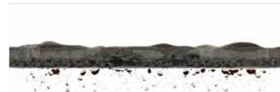
Conventional Flat Screen Solids Impede Fluid Flow
