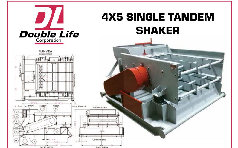
**DLC 4X5 SINGLE TANDEM** Shale Shaker has been designed to provide extended service life in all drilling related applications for which it was designed. Each unit is constructed of A-36 and/or 316ss plate built to proven oilfield specifications. The vibrating assembly can be powered by an electric motor or a hydraulic motor.
