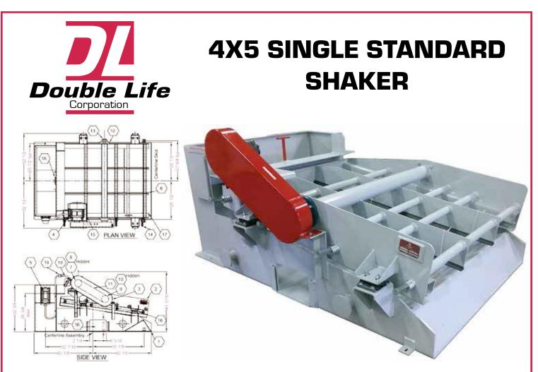
**DLC 4X5 SINGLE STANDARD** Shale Shaker has been designed to provide extended service life in all drilling related applications for which it was designed. Each unit is constructed of A-36 and/ or 316ss plate built to proven oilfield specifications. The vibrating assembly can be powered by an electric motor or a hydraulic motor.
